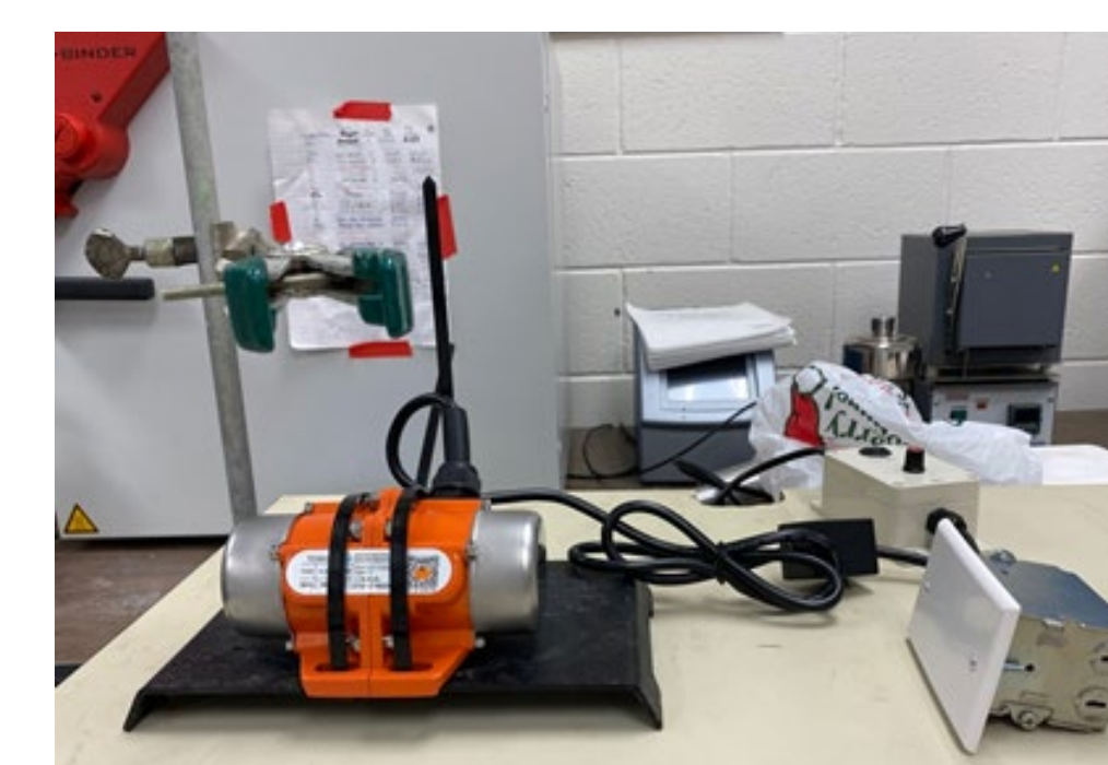
Figure 8: Experimental apparatus depicting vibrational motor, controller, and laboratory stand.
