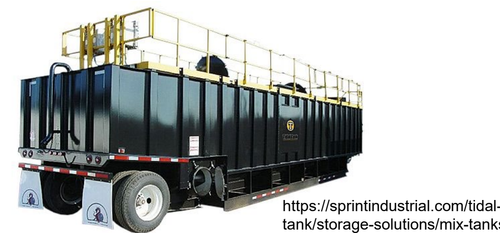
Figure 3: Frac tank for mixing
