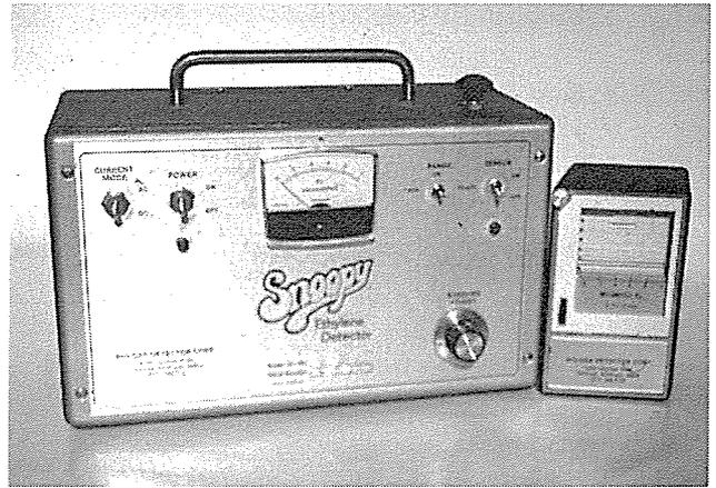
“Snoopy” – a device for measuring ethylene content of fruit under field conditions.
