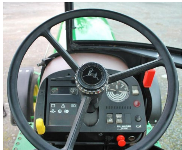
Figure 7. Indicator gauges as seen from operator's chair on tractor. Photo credit: www.flickr.com/photos/peterm7/4022045713/
