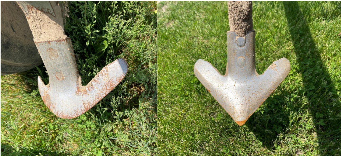
Figure 3. Side-by-side comparison of field cultivator shovels. The shovel on the left is worn with rounded blades and needs replacement. The shovel on the right is newer with sharper, even blade widths. Photo credit: Jonathan LaPorte, Michigan State University Extension
