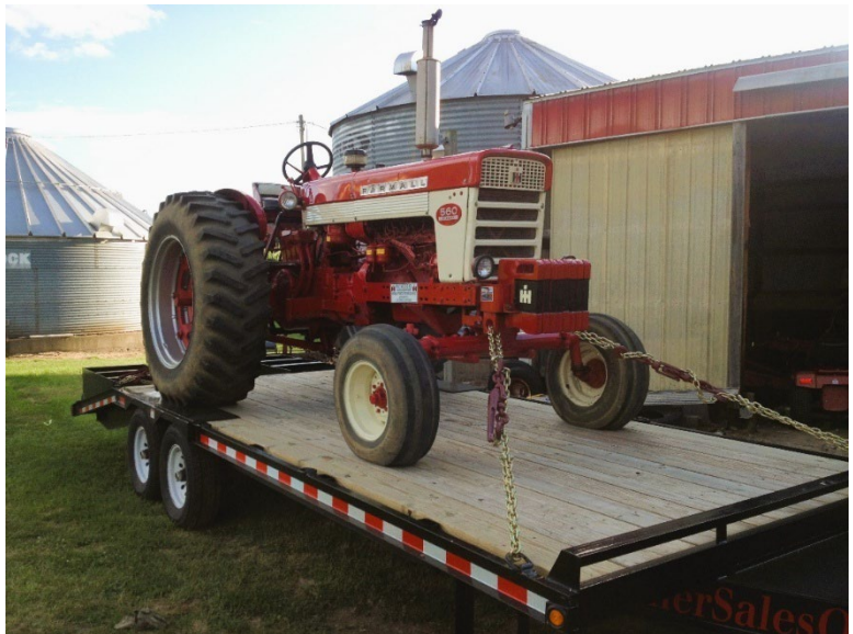
Figure 13. Tractor in the process of being secured to a flatbed, deck-over trailer with chains and lever binders. Photo credit: Jonathan LaPorte, Michigan State University Extension.
