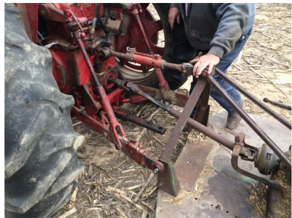
Figure 9. Hydraulic controlled three-point hitch connected to implement and power take-off (PTO) shaft. Photo credit: Jonathan LaPorte, Michigan State University Extension.
