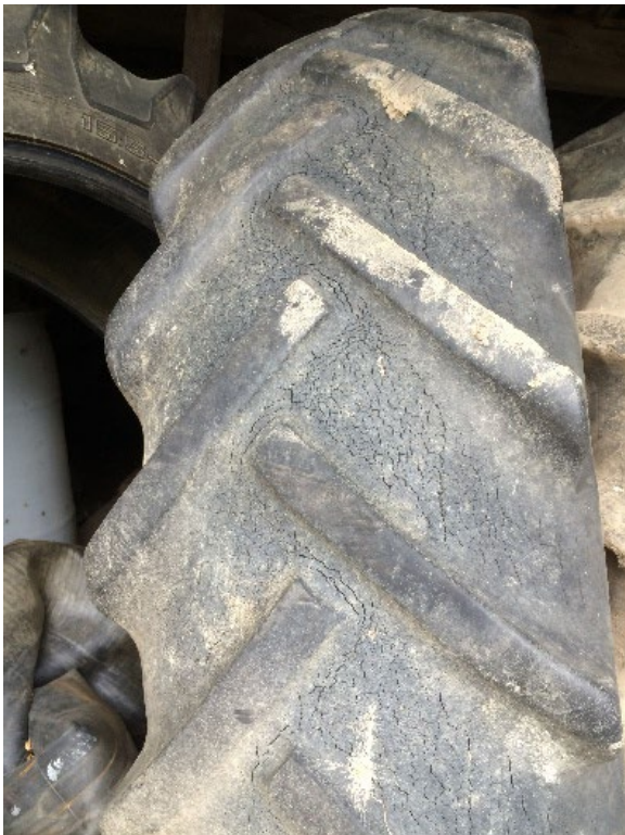
Figure 4. Tire with worn lugs and cracks in between lugs. Photo credit: Jonathan LaPorte, Michigan State University Extension
