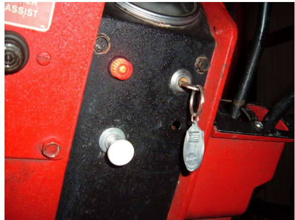
Figure 8. Brake light (red) engaging when clutch pedal is depressed. Photo credit: Jonathan LaPorte, Michigan State University Extension.
