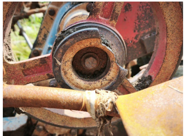
Figure 6. Broken pulley on a farm implement. Photo Credit: https://www.istockphoto.com/photo/close-up-of-broken-and-rusty-metal-pulley-on-agricultural-machinery-detailed-texture-qm2271736784-684183050
