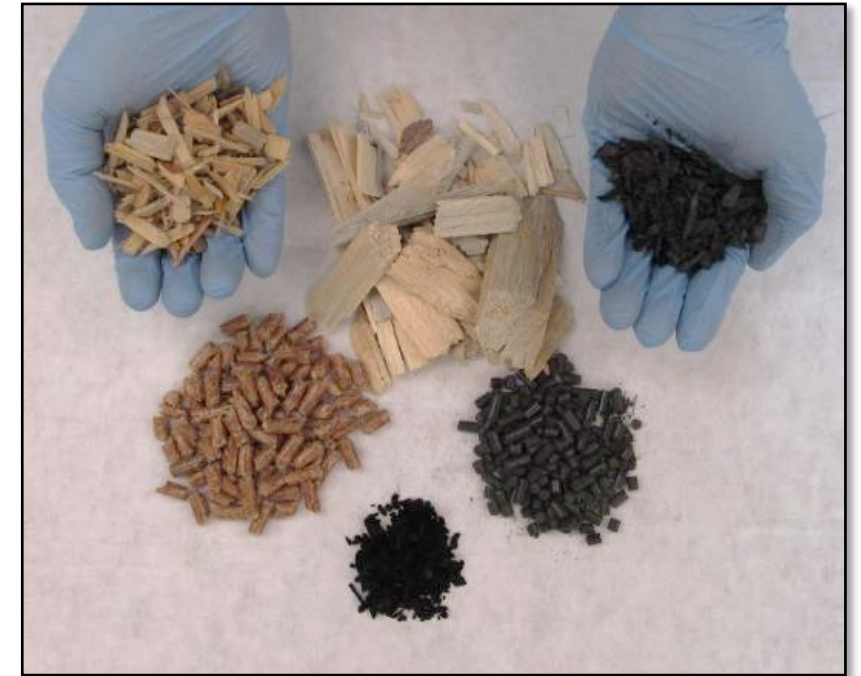
From top left: dry microchips, pulp chips, raw biochar, biochar pellets, activated carbon from biochar, and wood pellets.
