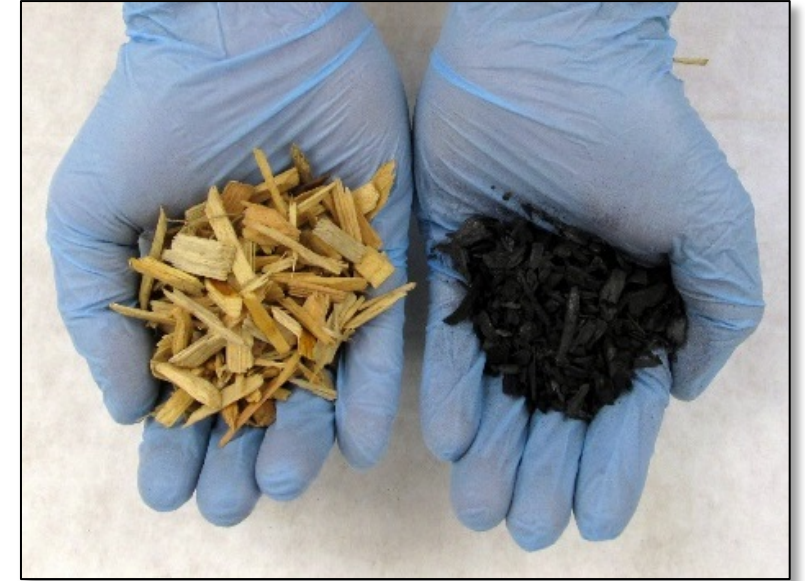
Chips and biochar produced from biomass harvested from White River National Forest.
