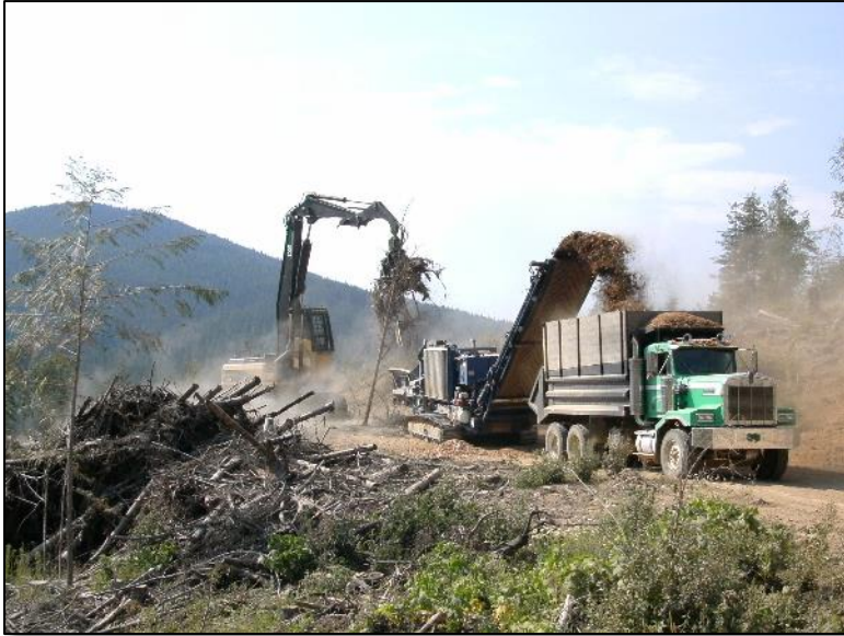
Harvesting woody biomass in Idaho to fuel cogeneration of heat and power.
