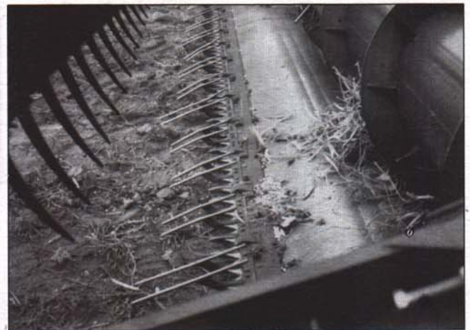
Vine lifters lift leaning plants and low-hanging pods above the sicklebar
