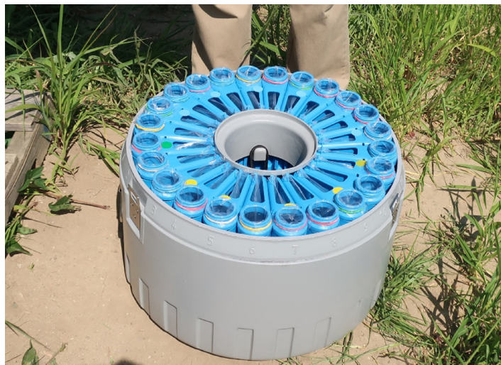
Figure 1- An automated sampler can perform flow-proportional or time-proportional sampling.
