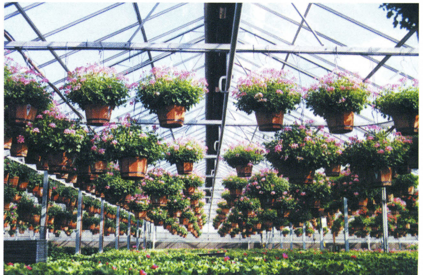
Growers find that with the uniformity of infrared heat, multiple layers of hanging baskets, bench crops, and floor crops can be safely grown in the same greenhouse.
