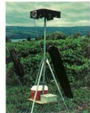
Photo 45. Auditory frightening device.
