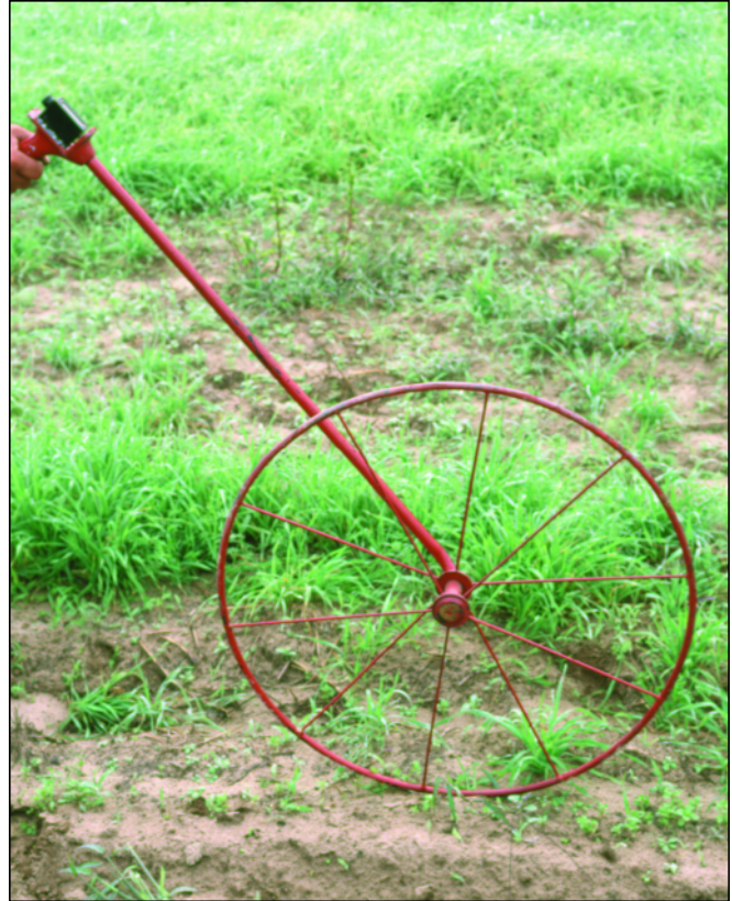
Fig. 7. This measuring wheel is used to easily measure distances for making a vineyard sketch. It records on a counter in the handle the number of rotations of the wheel as it is rolled along the ground. Each rotation is 6.6 feet.
