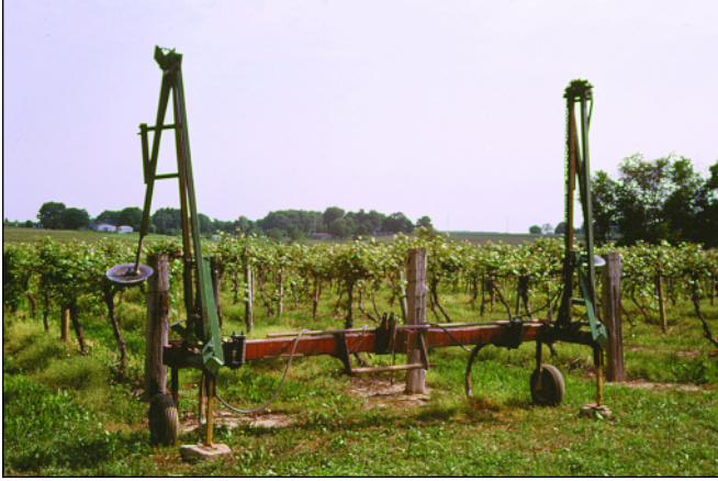
Fig. 2. This trailer field marker for planting grapevines on the Kerlikowske farm in Michigan uses two cultivating teeth to make grooves in the soil. Meanwhile a hydraulically extended disk marks the location for the next pass of the tractor. (Kerlikowske Farm, Berrien Springs, Mich.)
