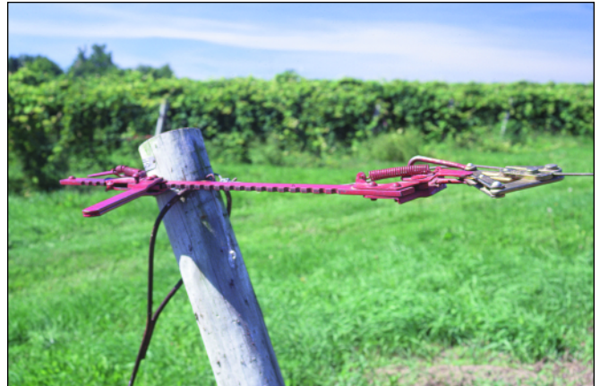
Fig. 36. A ratcheting wire tightener. A wire gripper has been welded on one end to reliably hold high-tensile wire.
