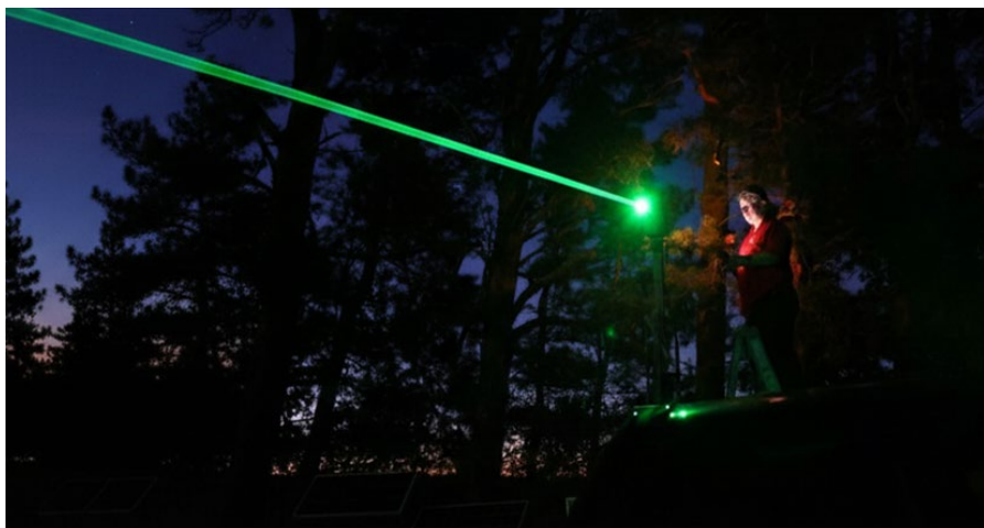
Figure 2. Automated green-laser bird deterrent installed at the Northwest Michigan Horticulture Research Center vineyard in Traverse City, Michigan. Photo by: Esmaeil Nasrollahiazar, MSU Extension
