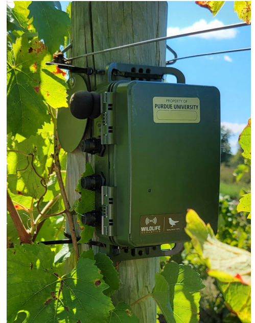
Figure 4. Passive acoustic recorder used to compare bird activity in the laser-protected and unprotected vineyard zones during Fall 2024.
