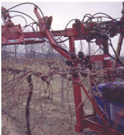
Fig. 12. Cane positioning on Concord vines using the fully-developed version of the device. Blum Farm, Lawton, Michigan.
