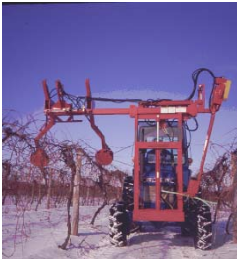
Fig. 11. Cane positioning being performed on a Concord vineyard. This unit can be quickly converted to a mechanical pruning operation. Baiers Farm, Bainbridge Township, Michigan.
