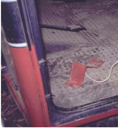
Fig. 17. A foot pedal override on a mechanical pruning device that can stop or reverse the action of the cutter bars. Oxley Farm, Lawton, Michigan.
