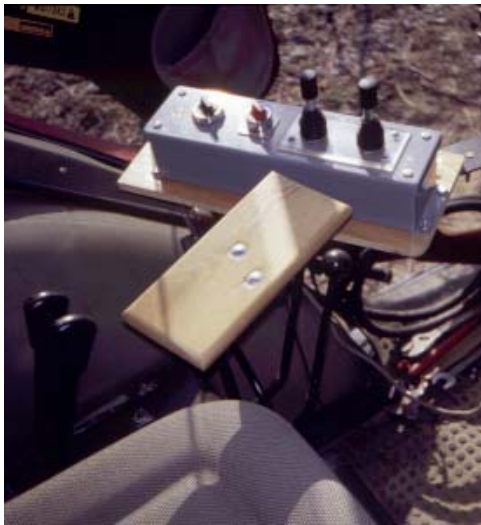
Fig. 15. Controls for a mechanical pruning device that promote ease of operation. Blum Farm, Lawton, Michigan.
