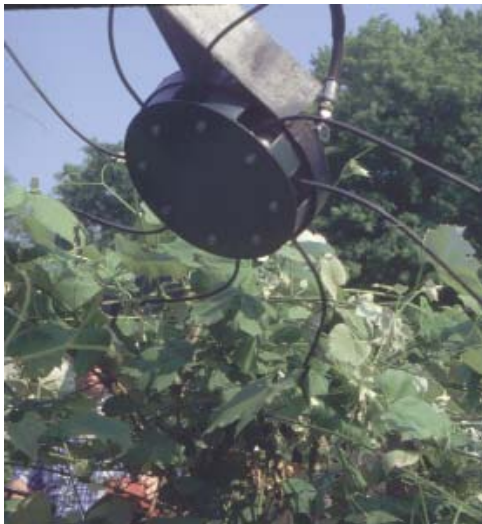
Fig. 13. Mechanical shoot positioning Concord grapevines with an MSU-Ag Engineering prototype at Southwest Michigan Research and Extension Center, Benton Harbor, Michigan.
