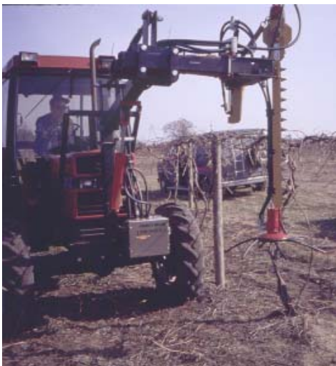
Fig. 16. Mechanical pruning device showing the aggressive orientation of the tines on the cutter bar as they point towards the trellis. Blum Farm, Lawton, Michigan.
