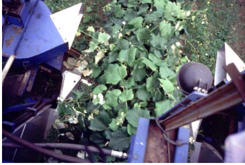
Fig. 4. Top view from a grape harvester being used to adjust crop size on Concord grapevines in mid-July. Green berries are somewhat visible on the conveyor belt and ground. Mihelich Farm, Teapot Dome, Michigan.
