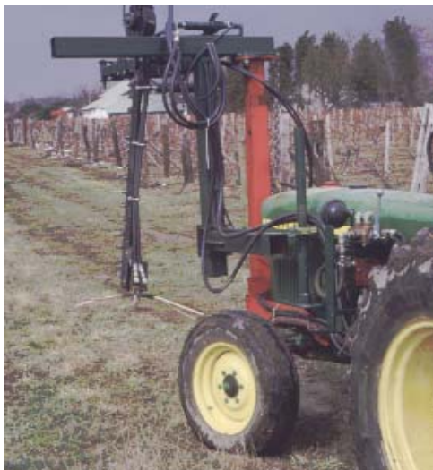
Fig. 8. A prototype mechanical pruning device constructed by the MSU Department of Ag Engineering. It features a dual-action cutter bar and rotating tines at the base of the cutter bar.
