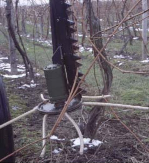
Fig. 9. A close-up of the rotating tines at the base of the cutter bar of an MSU prototype mechanical pruning unit. These tines move canes out from under the trellis into the path of the cutter bar.
