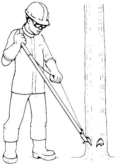
Figure 3.14. The tree injector offers a precise way of introducing pesticide into the trunks of well developed brush or trees.
