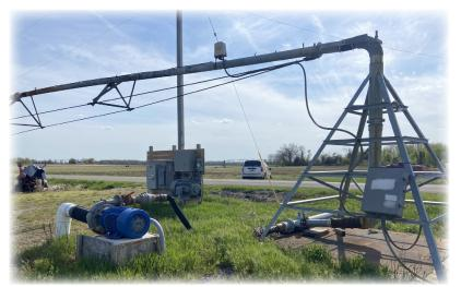
Irrigation well for a center pivot system. Photo: Lyndon Kelley, MSU Extension.
