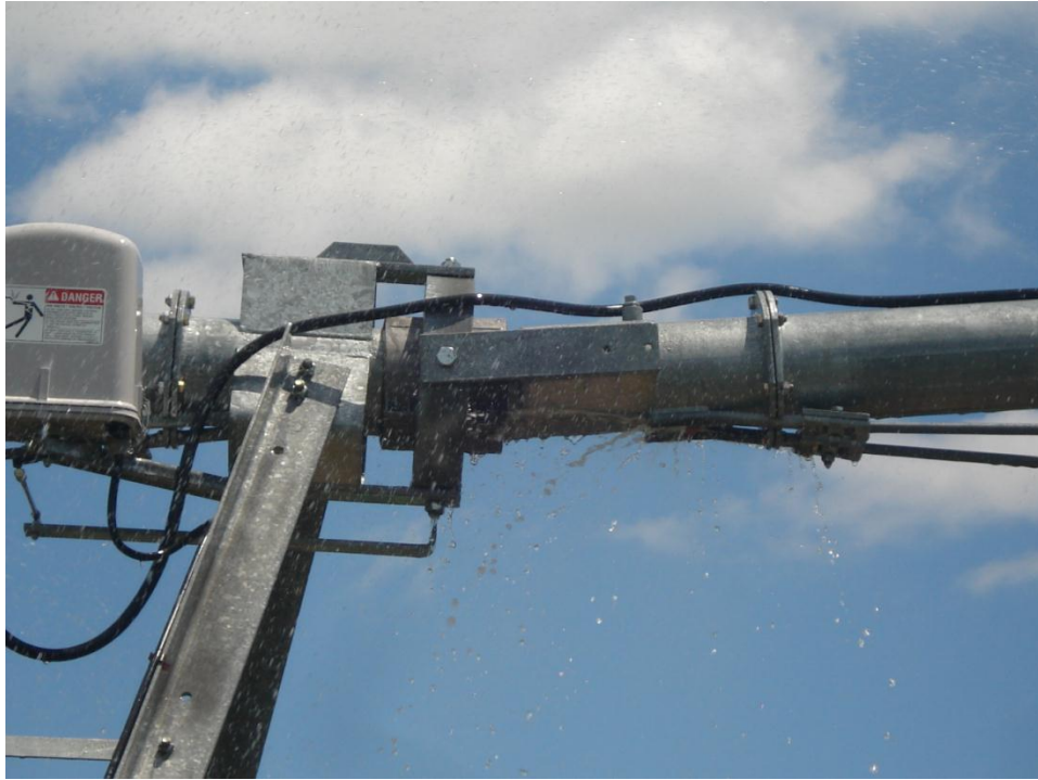
Figure 14. Water leaking from the lateral joint on the center pivot line.
