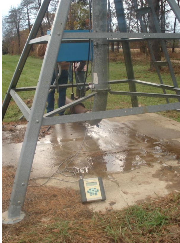
Figure 12. Using the Ultra-sonic flow meter to measure flow rate through the system.
