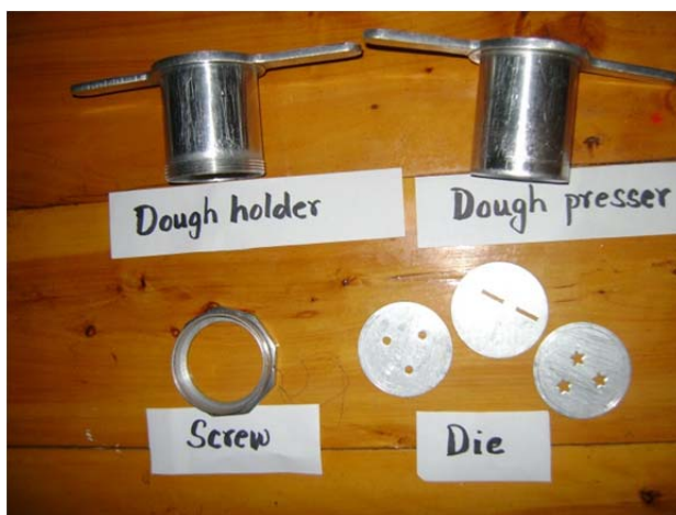
Figure 3– Elements of the Hand Held Cold Extruder
