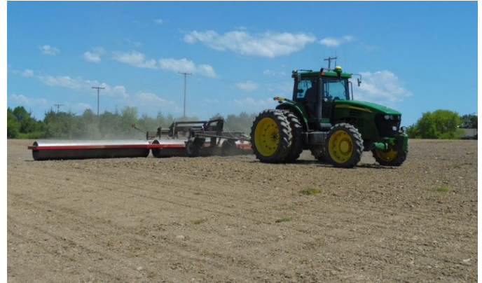
Figure 7. Large land roller operated under ideal conditions prior to soybean emergence. Mike Staton, MSU Extension.
