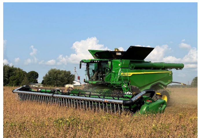
Figure 6. Combine equipped with a draper header and an air-assisted reel. Mike Staton, MSU Extension.
