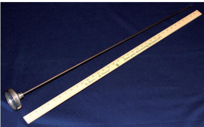
Photos 7a and 7b. Long-stem thermometer (available commercially as “compost” or “windrow” or “hay” thermometer) is used to monitor internal temperature.
