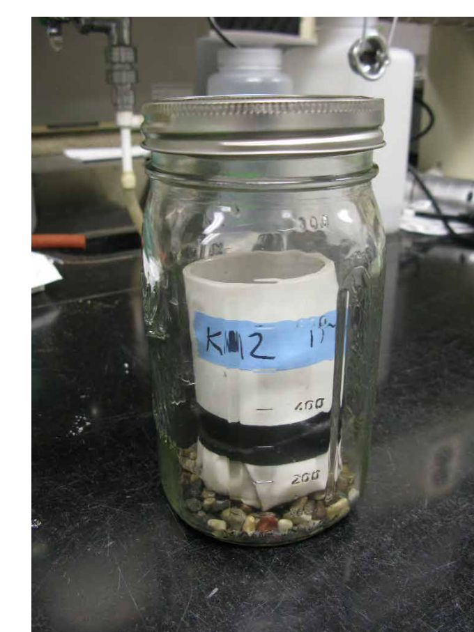
Figure 4 . Incubation chamber utilized by team for studying the effects of increasing cover crop diversity on microbial populations and weed seed decay (Tiemann and Renner).
