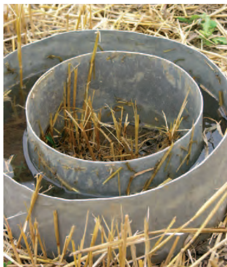
Water infiltration device to test how quick water moves into soil in the field. This is a good indicator of soil biophysical quality.
