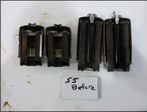
Cross section of fuel filters from Tractor 1 before the test burn. Photo courtesy of Paul Gross.
