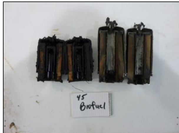
Cross section of fuel filters from Tractor 2 after the test burn. Photo courtesy of Paul Gross.
