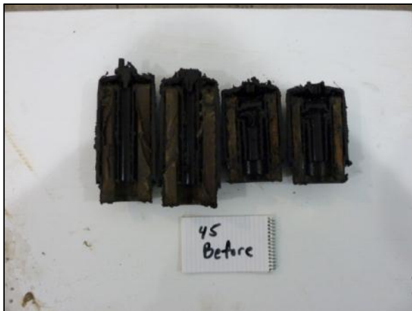
Cross section of fuel filters from Tractor 2 before the test burn. Photo courtesy of Paul Gross.
