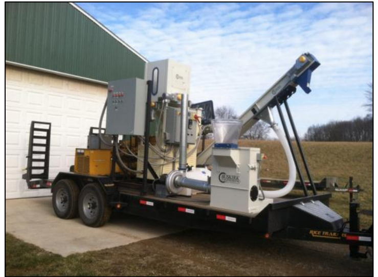
Portable pellet mill constructed for this project. Photo courtesy of Dennis Pennington.
