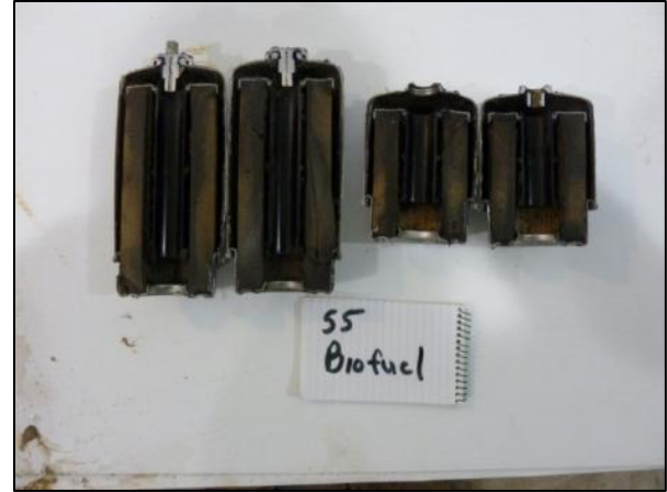
Cross section of fuel filters from Tractor 1 after the test burn. Photo courtesy of Paul Gross.
