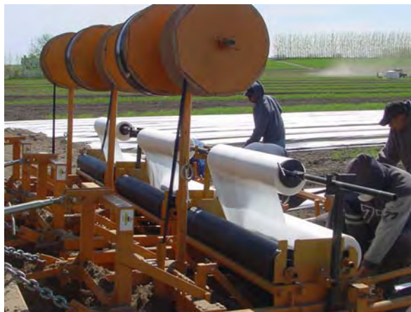
Figure 1. Applying plastic mulch and drip tape in 2005 using a three-row applicator. Clear plastic is used for low tunnels for earlier production
