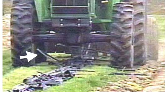
Figure 5. Tractor speed is too fast as indicated by the drip tape being pushed ahead of the baler (arrow).
