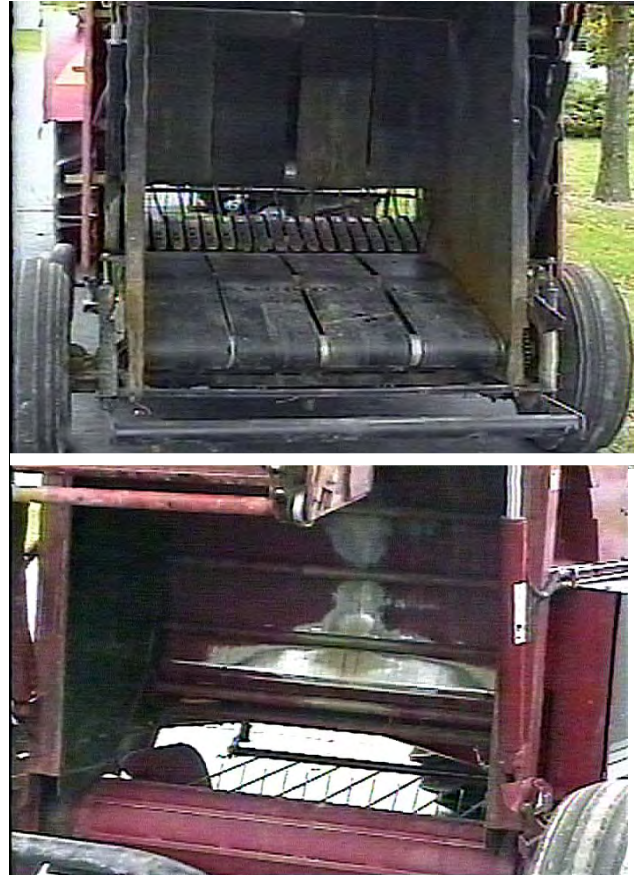
Figure 2. Belt baler (top) and chain baler (bottom) represent the two types of balers used to bale used plastic.
