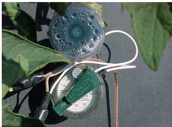
Figure 1. Tensiometer showing hard wire leading to solenoid valve. Tensiometer is set for 35 centibars
