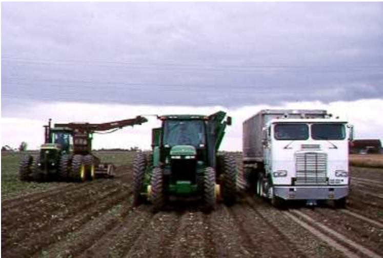
Tractor driven loader carts are also used to collect beets and transfer to trucks for transport.
