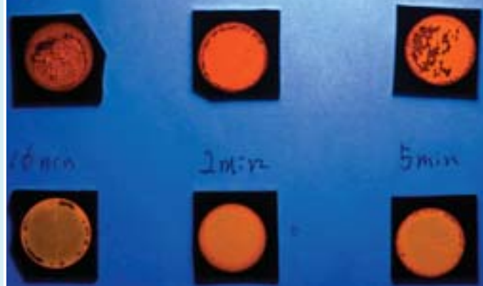
Far left: MAES scientist Evangelyn Alocilja uses nanomaterials to develop new types of biosensors to detect pathogens in food, water and animals. She recently developed a biosensor to detect Bacillus species and bovine viral diarrhoea virus. Left: Porphyrin solution. Above: Nanoporous silicon chip sensors have photo-luminescent properties.
