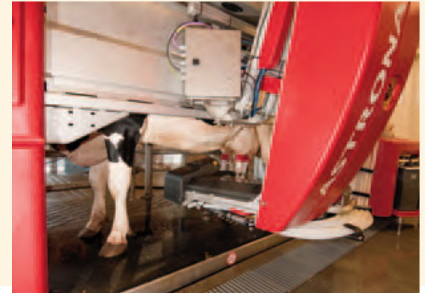
The new robotic milking machines at the W.K. Kellogg Biological Station pasture-based dairy were the second such installation in the state. The new dairy anchors education and outreach programs showing how ecological, social and economic principles can be evaluated on a small scale.
