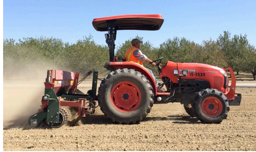
Seeding a wildflower planting with a mechanical drop seeder and cultipacker. Photograph: Katharina Ullmann, The Xerces Society.
