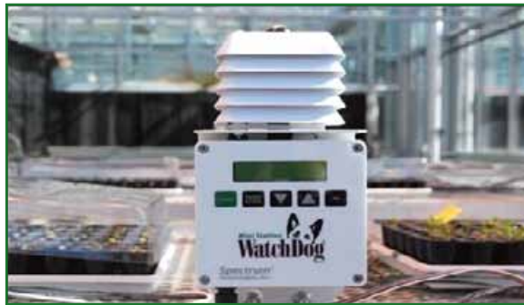
Figure 2. WatchDog weather stations contain light sensors and automatically calculate DLI.
