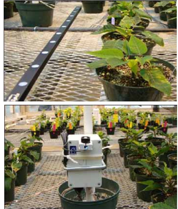
Figure 3. A light quantum sensor connected to a computer can measure and record instantaneous light levels throughout the day. These values can then be used to calculate the DLI received by the crops using Table 1.
