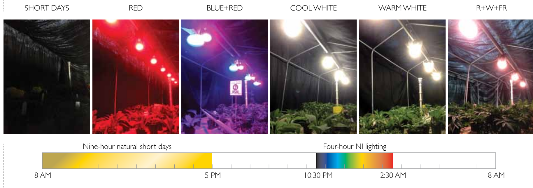
Figure 1. Experimental setup of a short-day treatment and night-interruption (NI) lighting treatments provided by red, blue+red, cool-white, warm-white, and red+white+far-red (R+W+FR) light-emitting diodes (LEDs).
