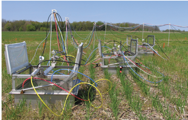
Automated greenhouse gas sampling chambers in a wheat field on the KBS Long-term Ecological Research site. These chambers measure nitrous oxide, carbon dioxide and methane emissions multiple times every day throughout the year, allowing researchers to accurately estimate greenhouse gas emissions. Photo: J.E.Doll, Michigan State University.
