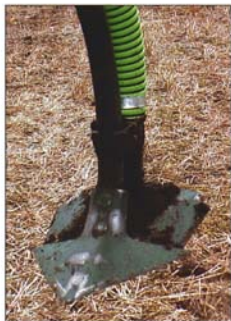
Winged injectors distribute the manure over a wide area.
