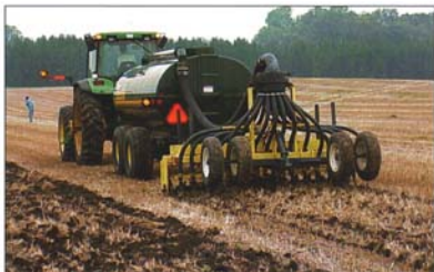
A rolling-tine aerator improves infiltration and nutrient recovery.
