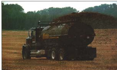
The faster travel speed of truck-mounted spreaders provides an advantage on longer hauls.
